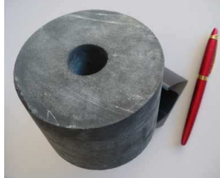
Figure 2: New materials developed from industrial wastes for solar power storage systems (PROMES, Perpignan)
