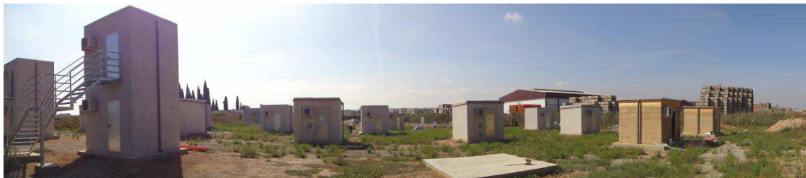
Figure 1: Test cubicles for comparing experiments of thermal energy storage materials for passive cooling (University of Lleida, Spain)
